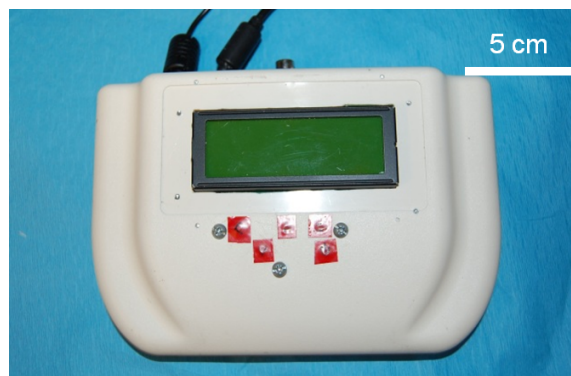
(b) Microcontroller control panel with push buttons and status screen.
